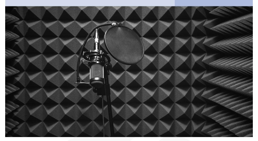
This light weight PU foam is a high performance sound barrier and which meets self extinguishing fire rating as per UL -94 standard.
