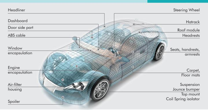
Polyurethane foam is an extremely versatile product used in countless applications worldwide. Polyurethane's mechanical properties can be isolated and manipulated through creative chemistry. This creates a number of unique opportunities to solve performance characteristics problems. It can have better hardness, better flexibility and better resistance.
