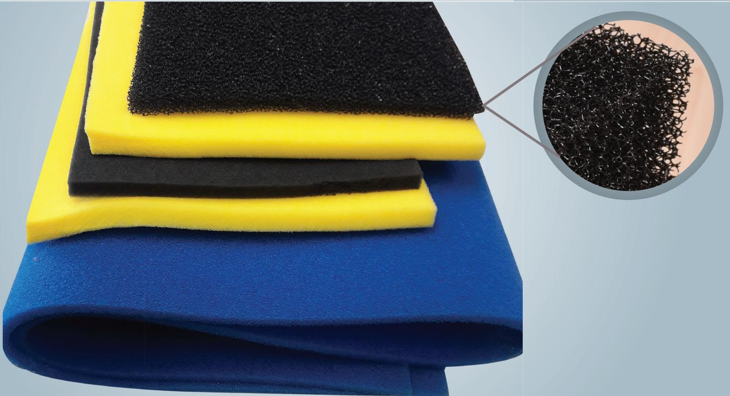
This Foam has 100% open cells made by thermal reticulation process. The Foam blocks are placed inside high pressure reticulation chamber for charging with gas to convert it in different PPI (pores per linear inch) depending upon the customer needs.
